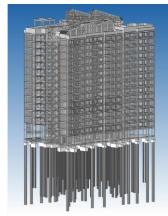
S4 – Fig 57 : Pile in relation to Building
